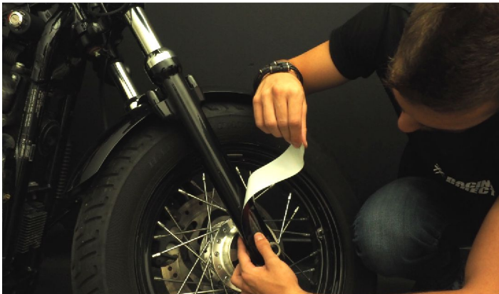
Clean the fork and apply the sticker.
