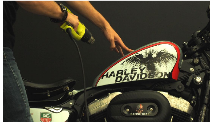
Fix the adhesive permanently with heat. Do not abuse the heat ... there is fuel in the tank!
